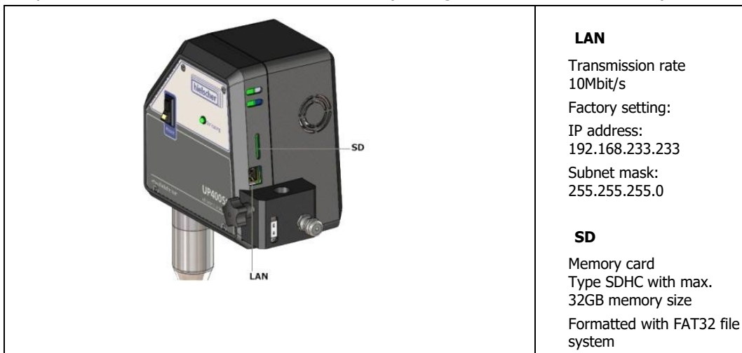
Figure 4-2 SD and LAN interface for memory card
